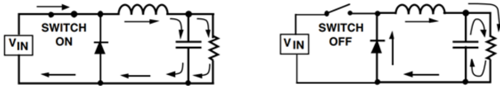
Figure 14: Buck Regulator Switching Current Flow Paths (Source: Texas Instruments - Literature SNVA559)(Permission Requested)
