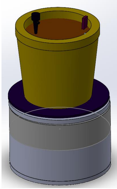
Figure 37: Moisture sensor installed on pot. Figure 38: Light sensors on edges of pot.
